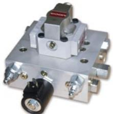
A single solenoid 'power to run' unit that will unload the test article in a controlled manner upon power failure. Designed to offer a high level of test article protection with symmetric loading actuators operating under closed loop servo control.
