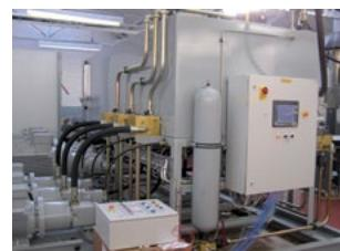
Specifically designed to be the heart of the aerospace test system. Units are available in a variety of sizes for virtually any application. The unit provides continuous hydraulic power to ensure your test runs exactly as planned, while offering a superior level of test specimen protection.
